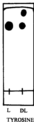
Fig. 2. TLC chromatogram showing the resolution of DL-tyrosine. Stationary phase: cellulose TLC plates. Mobile phase: methanol–formic acid– \beta -CD saturated solution of urea (7:1:2), pH 4.5.
